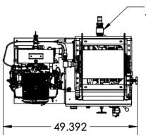
TK-PUMP CHECK VALVE - CAN BE RELOCATED TO TANK
