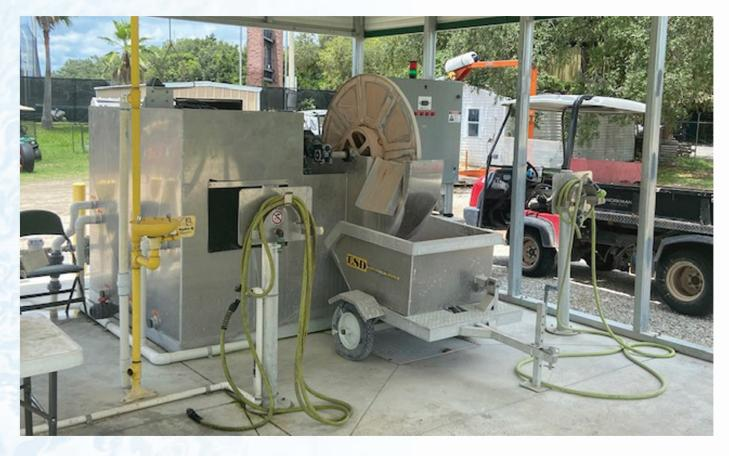
The Rotary Disc Vacuum System by ESD Waste 2 Water Inc. is designed to reduce moisture content in sludge by 85% or more. The RDV produces a cake material that can be easily transported for disposal.
