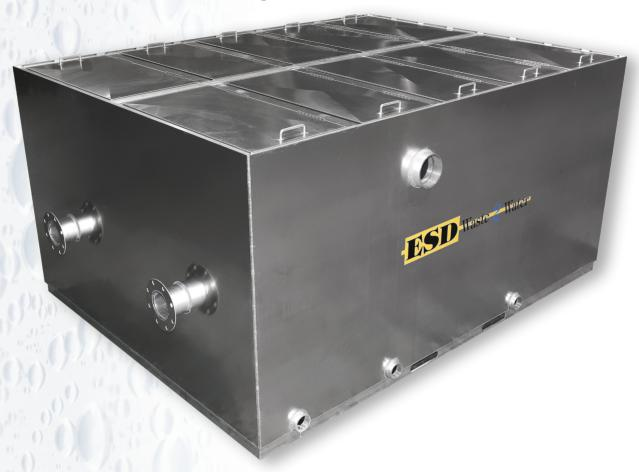
**ESD** Waste Water, Inc. manufactures a complete line of above ground, enhanced corrugated plate Oil/Water Separators designed to remove free and dispersed non-emulsified oil and settleable solids in accordance with API 421-90 @ flow rates up to 400 GPM. Typical applications are groundwater treatment, equipment / vehicle washing and bulk storage facilities.
