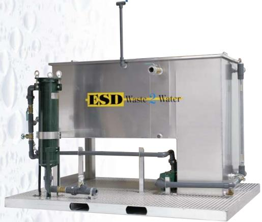
**ESD** Waste Water, Inc. manufactures a complete line of above ground, enhanced corrugated plate Oil Water Separators designed to remove free and dispersed non-emulsified oil and settle-able solids in accordance with API 421 @ flows from 10 to 250 GPM. Typical applications are groundwater treatment, equipment / vehicle washing and bulk storage facilities.
