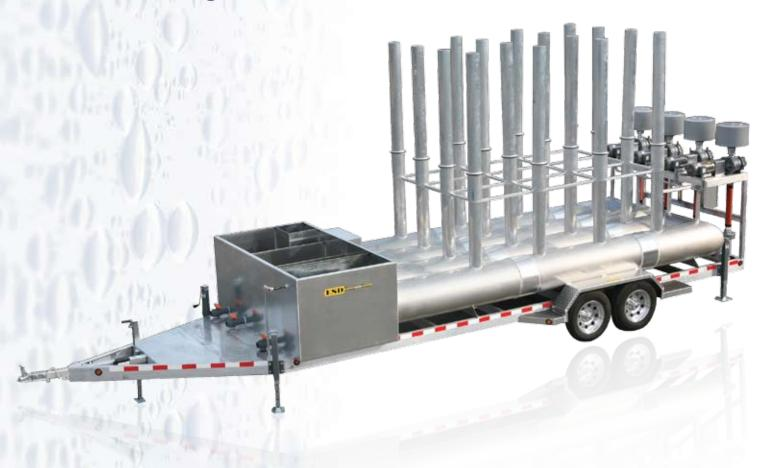
Waste Water, Inc.'s DW500 dewatering aerator is designed and constructed to efficiently remove hydrocarbons at flow rates up to 500 GPM and removal up 10,000 PPB. When operated within parameters the DW500 will remove hydrocarbons to FDEP discharge criteria making it ideal for dewatering sites. Equipped with a unique inlet settling tank, solids are removed before the treatment area and the design of the air delivery tubes allows for easy maintenance. Units are available for rental or purchase.
